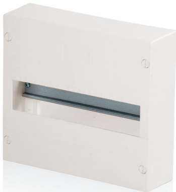
name N 12 A type IP 30 □ In 63A dimensions 225 x 250 x 70 number of modules 12 + 2 PE, N terminal 2 x 10
