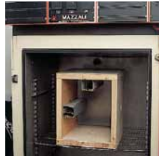
Cabin for age acceleration test.
