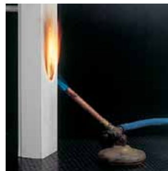
Apparatus for flame propagation resistance test.
