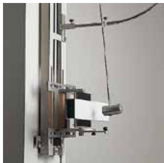
Apparatus for shock testing at room temperature.
