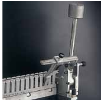
Apparatus for finger-removal and side-segment removal test.
