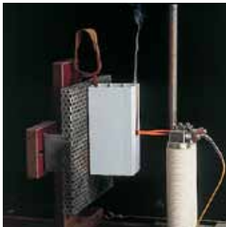
Apparatus for testing heat resistance (850° C) GWT.
